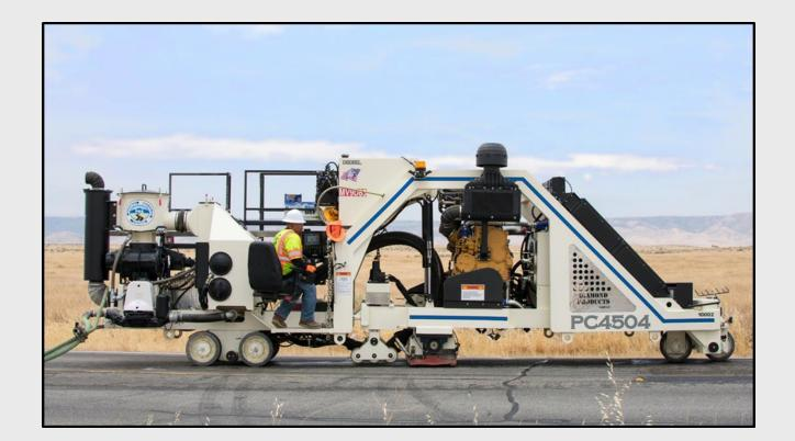
Is a "rigid" frame planer equipped with diamond tipped blades
