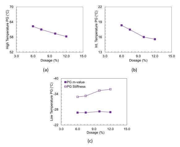
Figure 1. PG of 64-22 binder with increasing dose of REOB. (a) High PG, (b) Intermediate PG, and (c) Low PG. From Singhvi et al. 2020
