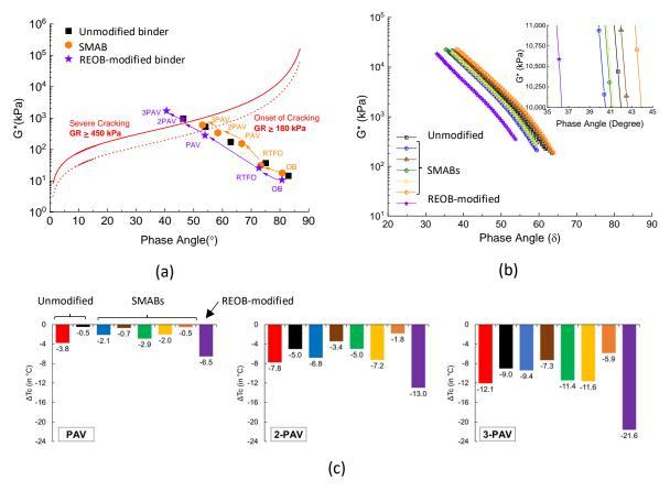
Figure 2. (a) GR, (b) Phase Angle at PAV aging condition, and (c) Tc results. From Singhvi et al. 2020. Modified
