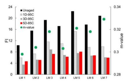
Figure 5. FI and binder m-value for mixes and respective binders. From Al-Qadi et al. 2019
