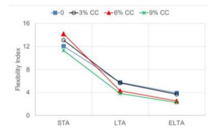
Figure 4. Impact on the FI of aging under different aging conditions (Short Term Aging [STA], Long-Term Aging [LTA], and Extralong-Term Aging [ELTA]) for mixes prepared with control and CC-type ReOB. From Ozer et al. 2016.
