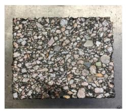
Figure 3: 9.5 NMAS SMA Section.
