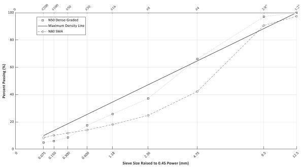
Figure 2: 0.45 Power Gradation Chart showing mix comparison.
