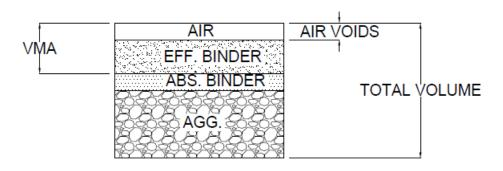
Figure 1. HMA Volumetric Diagram.
