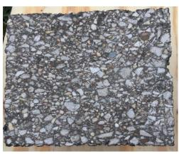
Figure 4: 9.5 NMAS Dense-Graded Mix Section.
