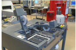
Figure 4. Specimens in the Wheel Tracking Test (Stuart et al., 2001).
