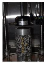
Figure 1. A Specimen in the Flow Number Test (Al-Qadi et al., 2012).
