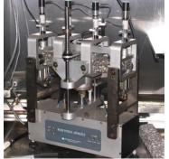
Figure 3. A Specimen in the Beam Fatigue Test (Flexural Fatigue, 2018).
