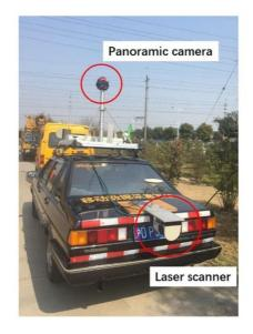
Figure 2. Set up of laser camera and panoramic camera used in the study (Wu, H. et al., 2019).
