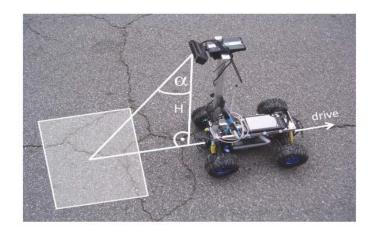
Figure 6. shows a remotely controlled sensing Robot vehicle for the experiment (Koch et al., 2013)
