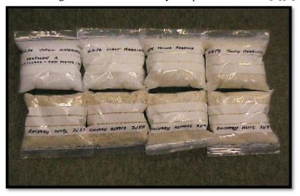
Figure 1. The color change in HDPE can be clearly seen after 10 process cycles. Virgin material (top left), material injection molded, and re-granulated 10 times (bottom left).
