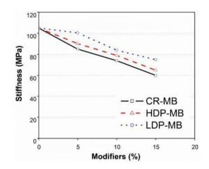
Figure 11: Stiffness of CR, HDPE, and LDPE modified binders at -10 °C [16]
