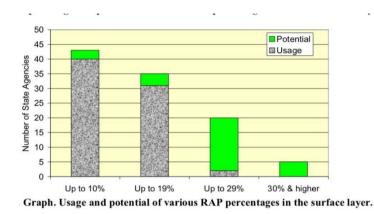
Figure 14: Usage and Potential usage of various RAP percentages in Surface layer [20]
