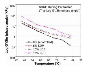
Figure 8: Effect of temperature and percentage of LDPE on rutting parameter of LDPE-MB [16]
