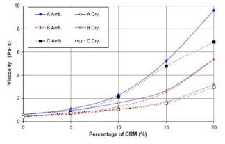
Figure 5: Viscosity of Experimented CRM Binders % [14]
