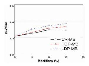
Figure 12: Rate of change in creep stiffness (mvalue) at -10 °C for CR, HDPE, and LDPE modified binders [16]
