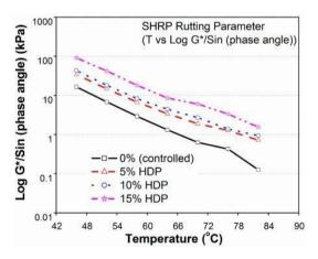
Figure 9: Effect of temperature and percentage of HDPE on rutting parameter of HDPE-MB [16]
