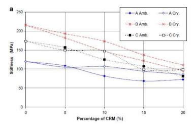
Figure 6: Stiffness of Experimented CRM Binders % [14]
