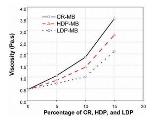
Figure 7: Viscosity of controlled and CR, HDPE, and LDPE modified binders at 135°C [16]
