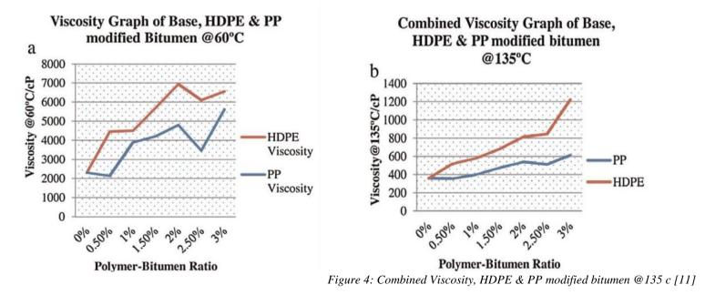
Figure 3: Combined Viscosity graph of base, HDPE & PP modified bitumen @60 c [11]
