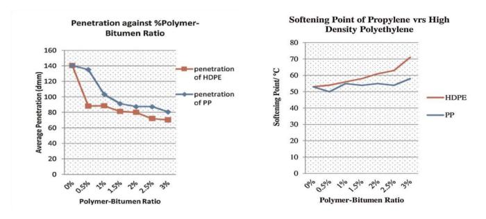
Figure 1: Penetration Graph of HDPE vs PP [11]
