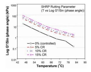
Figure 10: Effect of temperature and percentage of CR on rutting parameter of CR-MB [16]
