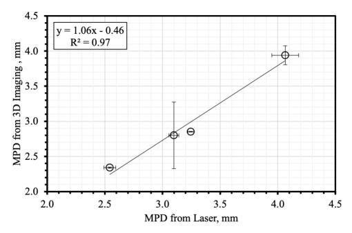
Figure 6. The Correlation Between the 3D Image-based Method and the Laser-Based Method (Boz et al., 53)
