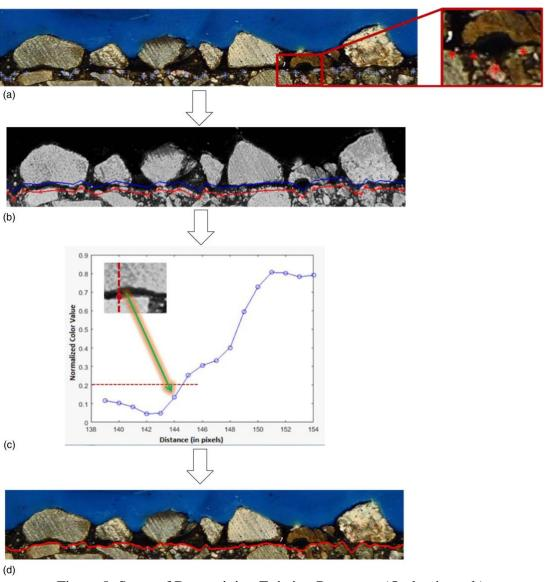
Figure 8. Steps of Determining Existing Pavement (Ozdemir et al.)
