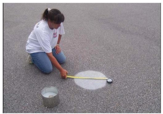
Figure. 1 The Sand Patch Test Being Done in the Field (Minnesota DOT)
