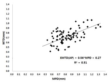
Figure 3. Correlation of Sand Patch Test and Portable Laser Profiler (Kim et al., 1586)
