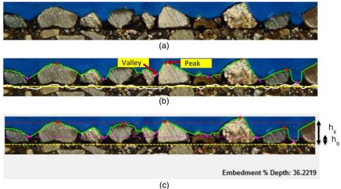
Figure 9. Steps of the peak and valley method: (a) original image; (b) finding peak and valley points—existing pavement's determination; and (c) embedment depth calculation (Ozdemir et
