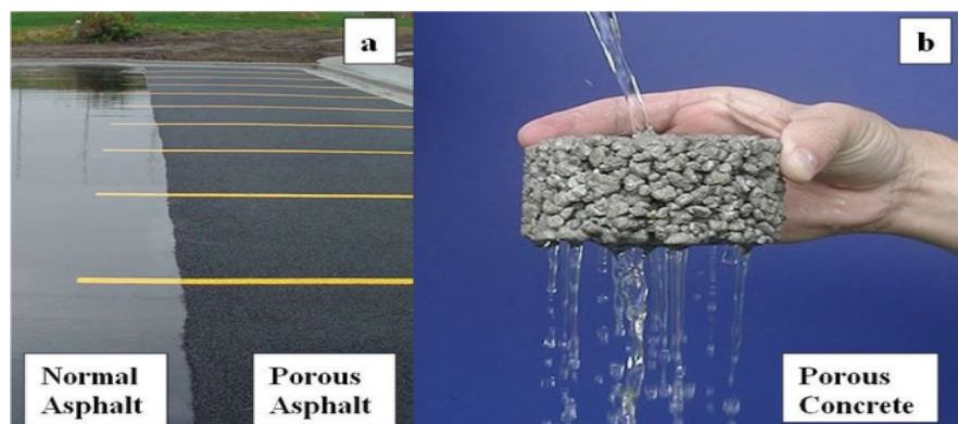
Figure 1: Normal and Porous Asphalt (NAPA, 2012); b) Porous Concrete (Hall, 2012)
