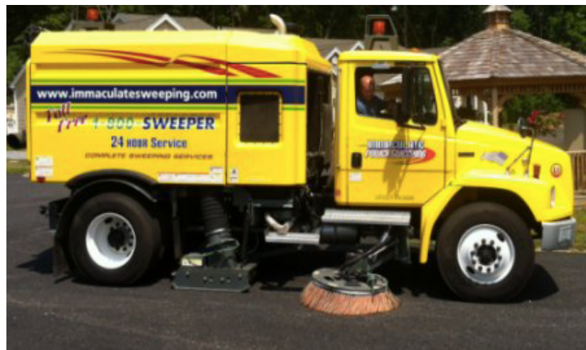
Figure 3: Porous Pavement Commercial Cleaning Unit
