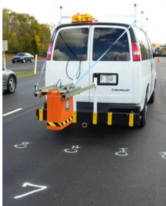
Figure 2: Typical GPR setup on a van
