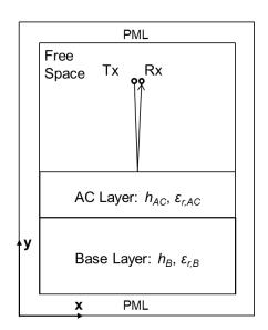
Figure 2 the three-phase asphalt mixture numerical model.
