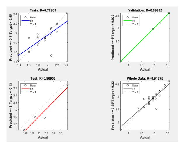
Figure 4. Predicted V Actual Rutting Depth for Training, Validation, and Test Data
