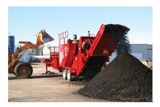
Figure 2) Shingles being grinded down (16)
