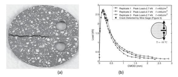
Figure 6 (a) Typical fractured DCT specimen (Wagoner et al., 2005) (b) Typical test curve
