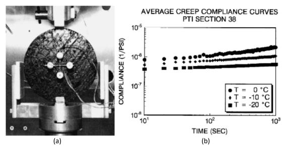
Figure 8 (a) IDT test setup and (b) typical creep compliance curves (Roque & Buttlar, 1992)
