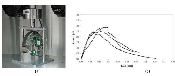
Figure 7 (a) SCB test setup and LLD extensometer, and (b) Typical plot of SCB test for three replicates (Marasteanu et al., 2012)
