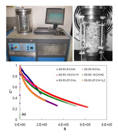
Figure 11 AMPT Apparatus and Specimen with Typical Test Results
