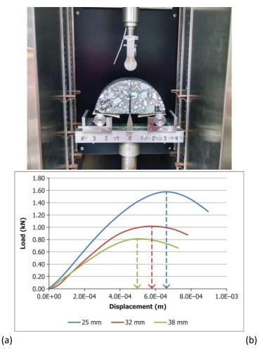
Figure 10 (a) LTRC - SCB test setup and (b) Typical test result
