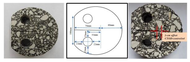
Figure 15 Modified DCT geometry and 1-cm offset CTOD for CDCT test (Chiangmai, 2014)
