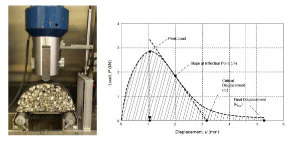
Figure 9 I-FIT setup and typical load vs. displacement plot
