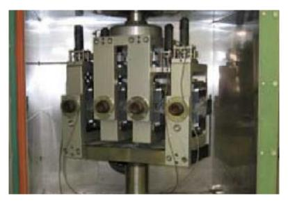
Figure 14 Four-point flexural beam fatigue test apparatus (Su et al., 2009)
