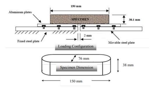
Figure 12 Texas Overlay Tester (OT) setup (Walubita et al., 2012)
