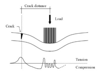
Figure 5 Bending Induced Mechanisms for Top-down Cracking
